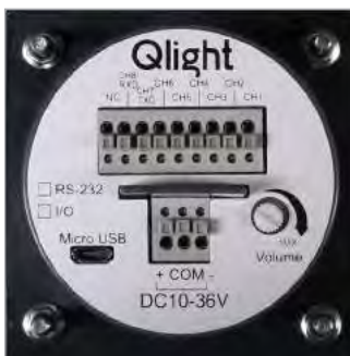
Terminal box for communication panel (back side)
