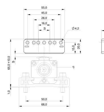
1) not included in scope of delivery, 2) Lateral offset, 3) Distance to BTL
